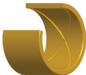
Bronze Bushed-S.A.E. 660 bronze with figure "8" oil groove
